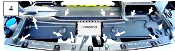
5. Depress the tab on the shutter body connector and disconnect. Repeat for the forward-facing camera (if equipped). Using a flathead screwdriver, or trim tool, pry the clip on the windshield wiper fluid hose (if equipped) fitting until it can pull out. Then pry up the harness clip attached to the top of the shutter housing. Place the wires toward the engine and free of the grill.
