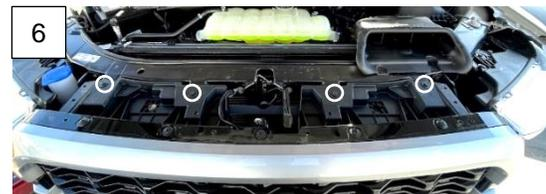
7. Directly under where the grill was mounted, there is a wiring harness along the top of the lower air dam. With the flathead screwdriver, or trim tool, remove the circled harness clips. Above the passenger frame rail, there is a large bumper connector that will need to be removed.
