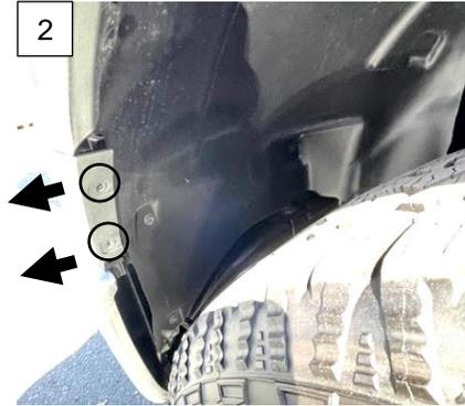
3. Once both sides are free, gently pull on the front of the grill trim piece away from the vehicle until it releases from the clips. Place aside. With the 8mm socket wrench, remove the two arrowed bolts that are on the bottom corners of the grill.
