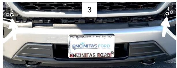
4. Open the hood. With the flathead screwdriver, or trim tool, remove the 12 arrowed plastic fasteners from the plastic radiator cover and place the cover aside.
