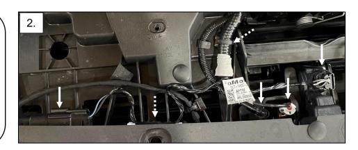
3. Fold up the rubber radiator shroud and remove the 4x bolts securing the top of the front grille using a 10mm. There will be 2 on each side.
