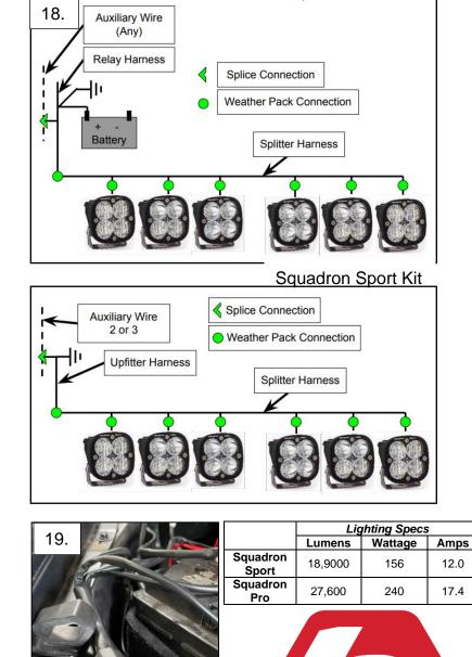
18. Place the large splitter harness to the lights with the main connector facing the passenger side of the vehicle. Plug in the Up-fitter or relay wiring harness to the splitter harness. Mount the grille when connected. Test lights before installing the grille hardware. If there is any confusion, use the diagrams on the right to show the difference in wiring between the Squadron Pro & Sport
