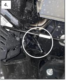
5. Using a 7mm socket, remove the 2x fasteners securing the fender flare. Repeat process on opposite side.
