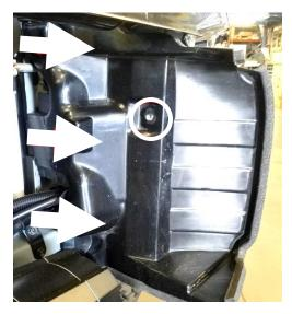
9. Locate the three bolts on the driver side Aluminum front bumper structure. The two circled in the picture below will be used to mount the bracket. With a 14mm socket wrench, remove the bolt closest to the center of the vehicle, then loosen the bolt right next to it until it is about 1/4" above the surface of the black plate.
