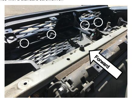
4. Underneath the front of the vehicle, remove six bolts with a 10mm socket wrench. Three are shown in the passenger side picture below.
