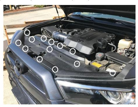
1. To remove the fasteners, gently press straight down onto the circular portion of the head until it is in the lowered position shown below.
