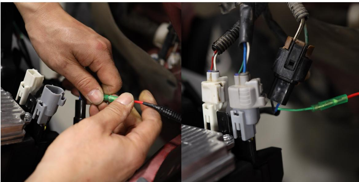
Connect the wires to the headlight accordingly. The red wire with the green connector goes to your INJ fuse, located in the fuse box under the hood. We recommend using a fuse tap (It's not included).
