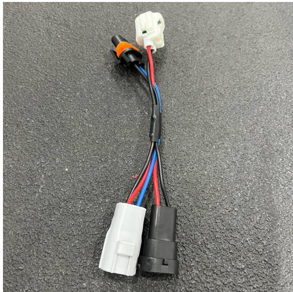
Some models need to use the supplied harness. Make sure all 4 connectors are plugged in to work properly.
