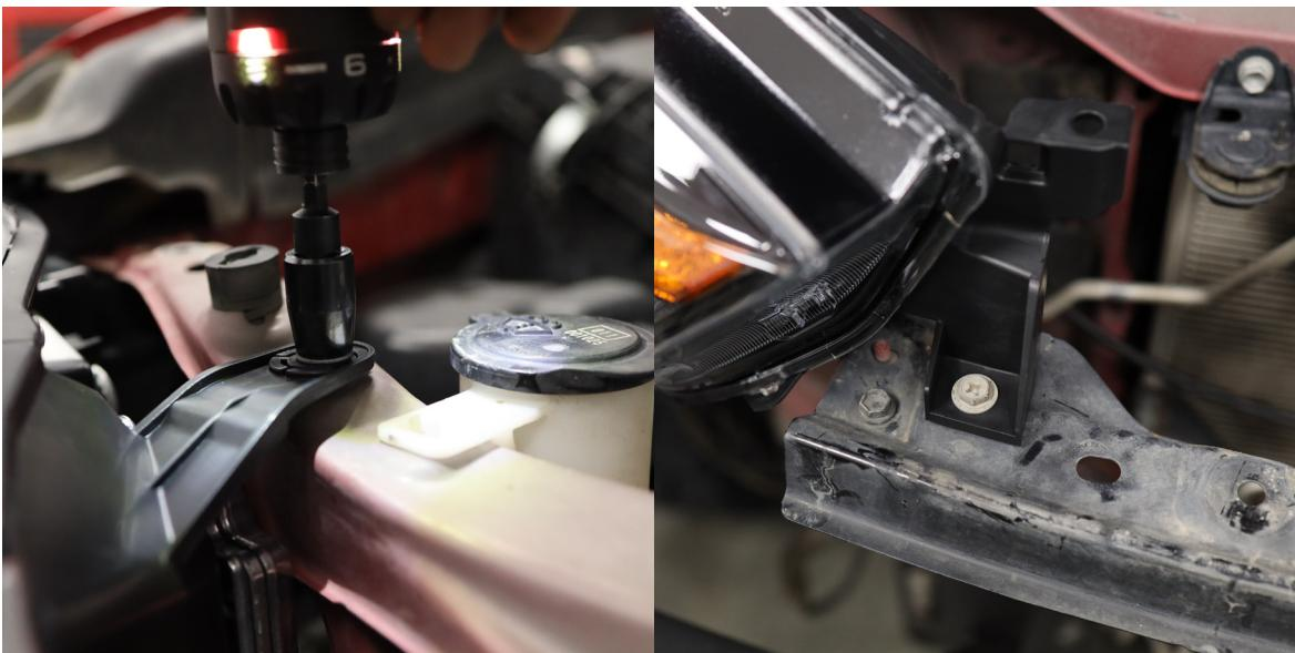
Attach the headlight using the factory screws and a 10mm socket tool.
