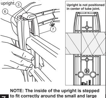
Tighten PT-Screws using a T-25 torx driver. starting in the middle of each upright, then the outer screws and lastly the remaining two to evenly tighten.
