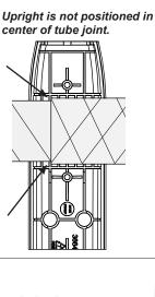
NOTE: The inside of the upright is stepped to fit correctly around the small and large diameter tubes. Tighten PT-Screws using a T-25 torx driver, starting in the middle of each upright, then the outer screws and lastly the remaining two to evenly tighten.
