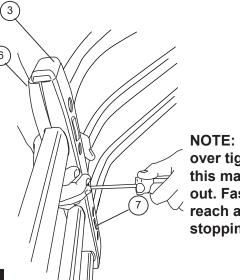
NOTE: Do not over tighten as this may strip out. Fastener will reach a noticeable stopping point.
