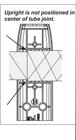
NOTE: The inside of the upright is stepped to fit correctly around the small and large diameter tubes. Tighten PT-Screws using a T-25 torx driver, starting in the middle of each upright, then the outer screws and lastly the remaining two to evenly tighten.
