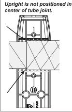
NOTE: The inside of the upright is stepped to fit correctly around the small and large diameter tubes.
