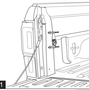
Install Pivot Brackets to upper two threaded holes on D-Pillar. Each bolt location will take two plastic spacers (4 total per bracket, as shown) under the bracket to properly space brackets.
