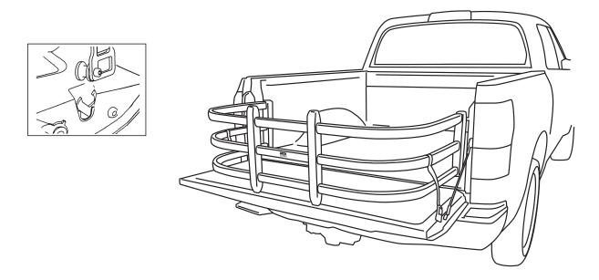
Pull tailgate release handle to release buckles from the tailgate.
