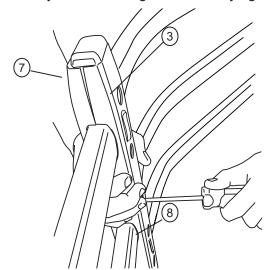
NOTE: Do not over tighten as this may strip out. Fastener will reach a noticable stopping point.
