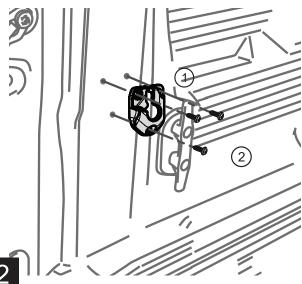
Fasten mounting brackets using the supplied self-tapping Phillips screws and torque to 30 in. lbs. If equipped with a bedliner, install mounting brackets over bedliner.
