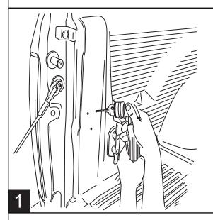
Using a power drill and 9/64" drill bit, drill through the existing dimple holes in sheet metal. If equipped with a bedliner, drill through bedliner.
