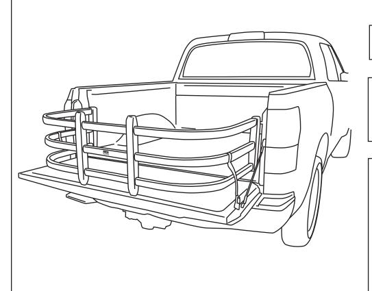
BEDXTENDER HD<sup>™</sup> shown assembled and installed on truck.
