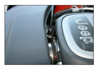
**4.** *A.*) Using the 10mm socket, remove the bolt that holds the stock intake system. *B.*) Loosen the hose clamp that holds the coupler to the throttle body.
