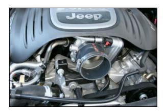
10. Install the coupler and two #60 hose clamps on the throttle body as shown. Do not tighten hose clamps. Fasten the factory breather hose to air conditioning line using the supplied zip tie.
