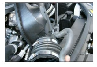
**6.** Slide the clip off of the intake tube that holds the breather line.
