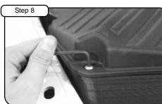
Tighten down cover housing using M6 button head screws and wavy washers.
