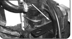
With 10mm socket, loosen bolt holding in radiator housing, install bracket "D" and re-tighten bolt.
