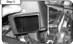
With screws provided (see step 6), install housing into vehicle. Make sure housing tab mounts up to bracket "D"
