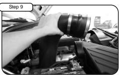
Install hi-temp & hump coupler with clamps provided to tube. Now install tube into vehicle. Do not tighten!
