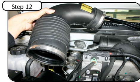
Step 12 Additional steps for Stage 2 installation: With 5/16 nut driver loosen both clamps on factory tube and remove.
