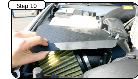
Step 10 Reconnect the MAF sensor harness. With 3 button head screws, install the housing cover. Tighten with allen wrench.
