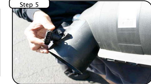
Step 5 Take out factory MAF sensor using the torx T-20 bit to unscrew bolts. Be careful in handling the MAF sensor.
