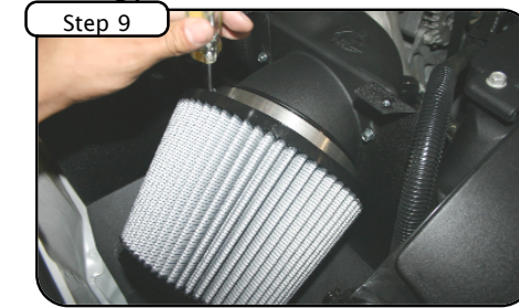
Step 9 Carefully install the 6" aFe air filter and tighten with 5/16 nut driver.
