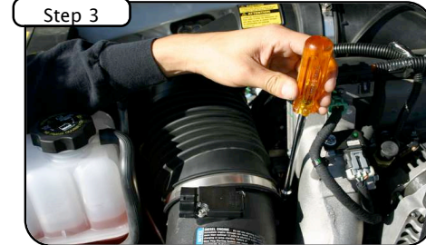
Step 3 Disconnect factory MAF sensor harness. With a 5/16 nut driver, loosen the factory tube from air box.
