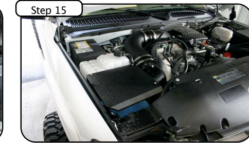
Step 15 Stage 2 installation is now complete. Check clamps and tighten periodically. Thank You for choosing aFe!
