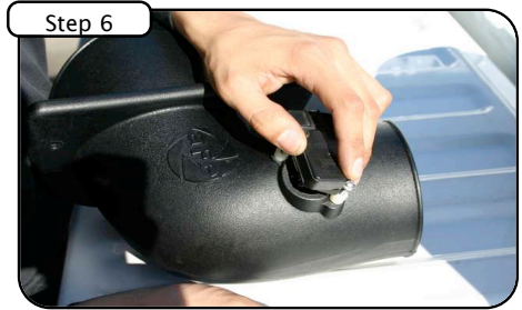
Step 6 Carefully put sensor into the new stage 1 tube with provided nylon spacers and sensor gasket. Slip gasket onto sensor with nylon spacers in between the tube and sensor. Tighten #8 screws with phillips screwdriver.
