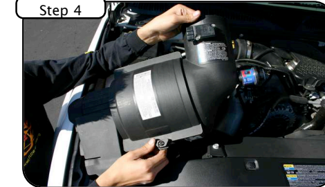
Step 4 Gently pull out whole airbox. Grab from MAF area, (not directly on MAF) and pull up. It is held in place with rubber grommets. Remove the airbox mounting plate bracket.
