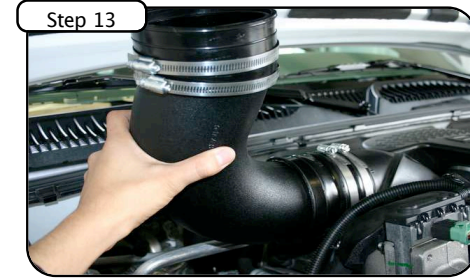
Step 13 Install 4 3/4" coupler onto tube, (05-00749) using clamps provided. Install 4 1/4" end of tube into coupler. Do not tighten.
