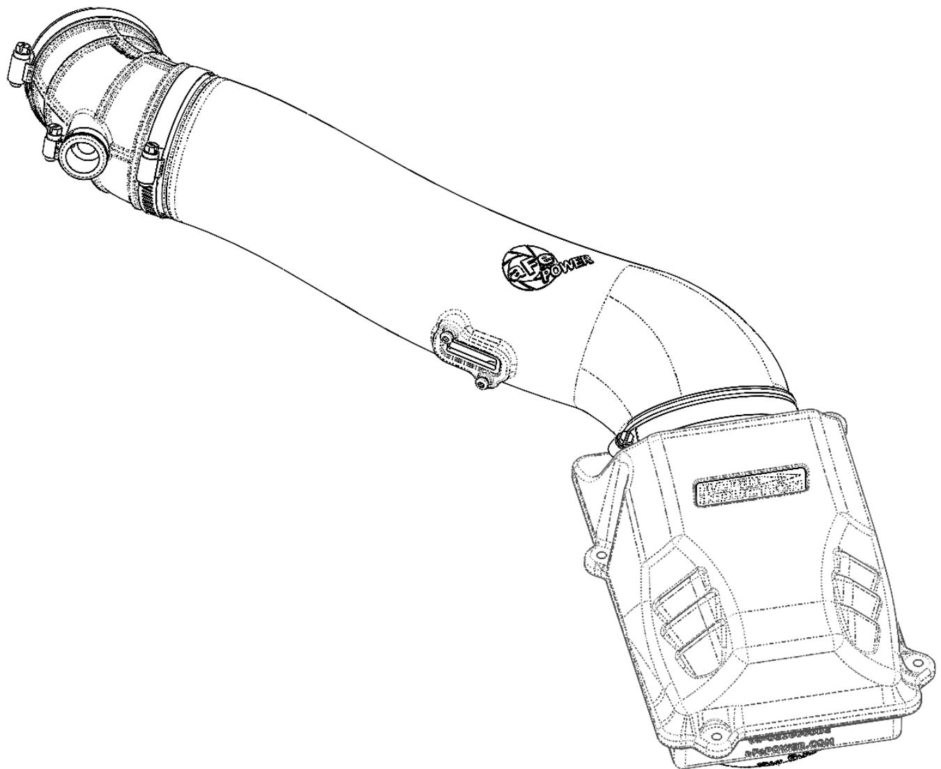
***advanced FLOW engineering*** Rapid Induction Cold Air Intake System
