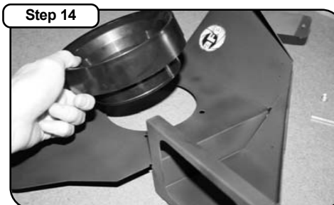
Install air filter adapter on aFe housing.
