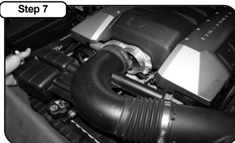
Disconnect air intake tube from throttle body.
