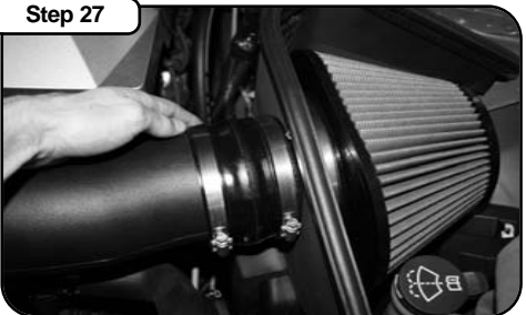
Connect aFe air intake tube to air filter adapter by sliding the loose coupling over to the right and tighten clamps.
