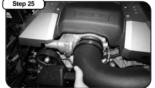
Connect aFe air intake tube to throttle body coupling.
