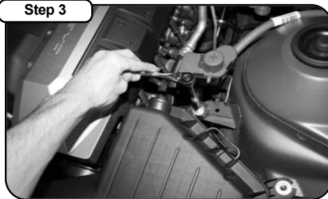
Remove nut from rear of air filter housing.
