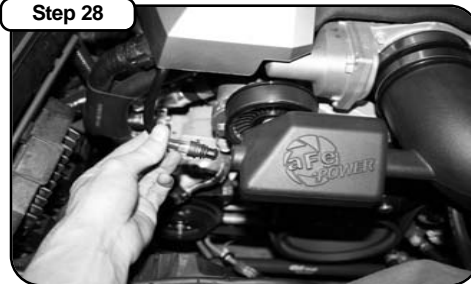
Insert breather line into aFe air intake tube.
