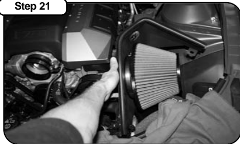
Install aFe housing into vehicle.
