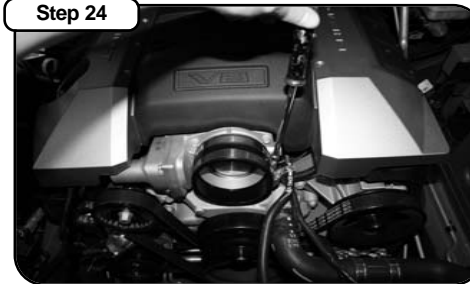
Install straight coupling and clamps (2) on throttle body inlet. Tighten clamp over throttle body.
