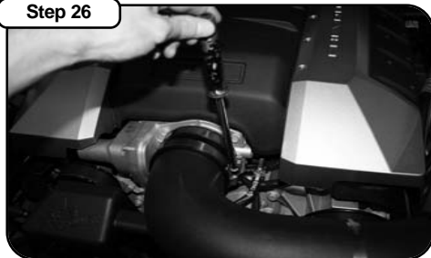
Tighten throttle body coupling clamps.
