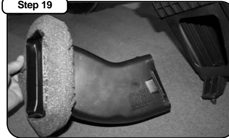
Remove air inlet duct from factory housing.
