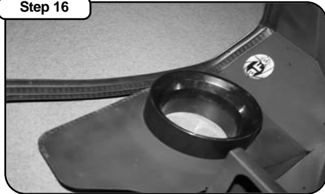
Install supplied trim seal on housing
