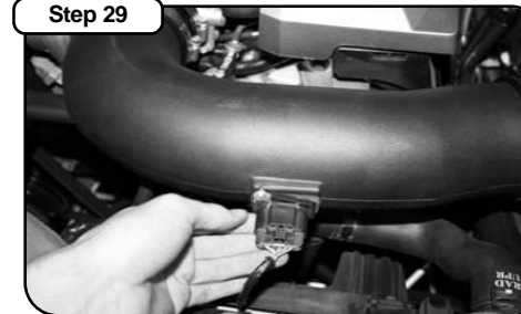
Plug electrical harness into MAF sensor.
