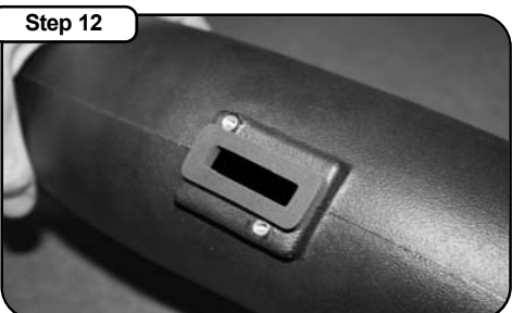
Remove white backing material and attach supplied gasket to aFe air intake tube.
