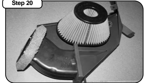
Insert factory air inlet duct into aFe housing.
