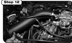
Remove large diameter vent hose still connected to the throttle body and small diameter vacuum hose, retain factory evap hose (closest to heat shield.) Replace removed hoses with hoses in kit and connect all hoses to intake tube; clamps are not necessari.
