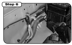
NOTE: (On 4Runner, disconnect ground wires on inner fender)
