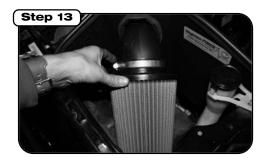
Install filter to intake tube. Re-position clamp and tighten. Do not use oil or grease. Reconnect factory harness to MAF Sensor
