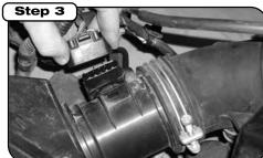
Unplug factory harness from Mass Airflow Sensor
