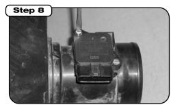
Remove factory Mass Airflow Sensor from factory air box.
