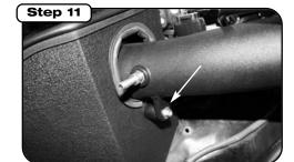
After tube is through housing install 7/16" trim seal to inside of housing hole. Use rubber isolation mount between tube bracket and heat shield. Tighten using M6 hardware provided.
