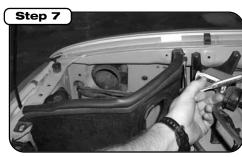
Install heat shield using provided hardware and reconnect ground wire to fender if applicable. Install 7/16" trim seal to top of housing.
