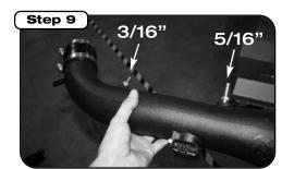
Install MAF sensor to new tube using M4 screws, spacers and gasket provided. Make sure spacers and gasket are between sensor and tube. Install brass nipples to tube and tighen.
