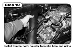
provided hose clamps and install intake tube. Use rubber isolation mount between tube bracket and heat shield.
