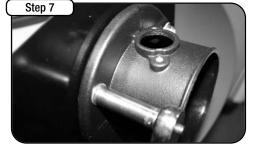
Insert Air filter adaptor in to housing using screws, nuts, and washers provided using 7/16" socket or wrench.
