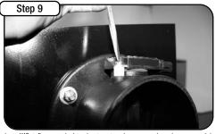
Insert MAS air flow sensor back into housing using nylon spacer, gasket and screws provided. Reconnect stack intake tube to Housing. Fasten securely using  $5/16^\circ$  nut driver. (*Make sure gasket and spacers are between tube and sensor*)
