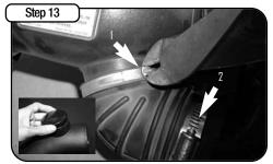
To install factory resonator, the stock clamp holding the resonator must be cut using a pair diagonal pliers. Using provided clamp, reinstall resonator onto tube.
