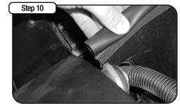
Install trim seal. Start with front end near radiator shroud.
