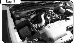
Complete Stage 2 kit installed. Make sure all clamps are tight and all components are secure. Check and retighten connections and filter after a few hours of operation. **Place the** included CARB EO Sticker on or near the intake system on a smooth, clean surface. E.O. identification label is required in passing the Smog Check Inspection.
