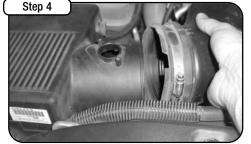
Loosen and separate stock intake tube from stock air box.
