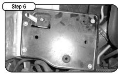
Remove (5) 10mm bolts as shown to remove air box pan.
