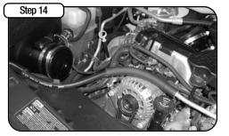
Install provided couplers. Be sure to install the small end of the tapered coupler to the turbo inlet housing. The remaining coupler must be installed with the smaller inner diameter attached to the heat shield, and the larger inner diameter will receive the Stage 2 tube. Install Stage 2 tube into couplers. Reposition duct clamps if additional clearance is necessary.
