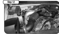
Complete Stage I kit installed for stage 2 instructions, continue on to steps 13, 14 and 15.
