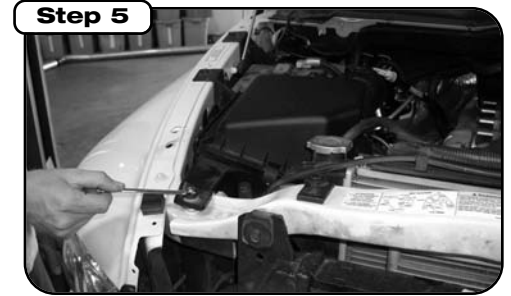
Step 5 Using 10 mm wrench, remove the bolt that secures the factory airbox to the radiator bulkhead.
