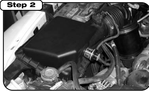
Step 2 Complete stock intake. Make sure that the engine has sufficiently cooled down prior to starting installation of this kit.
