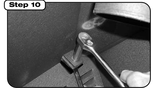
Step 10 Using provided bolts, locking nuts and washers on both sides of the bolt, fasten lower tab on heat shield and slotted hole to the existing rubber mounts. Be careful not to over-tighten, it is only necessary that the rubber mounts be slightly compressed. Fully tighten shroud.
