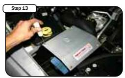
Install housing cover using button head screws provided. Tighten using 5/32" allen key.
