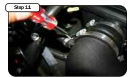
Tighten clamps on intake tube to plenum box with 5/16 nut driver. Place new vent hose onto tube and tighten clamp using 1/4" nut driver. (on Grand Cherokee models the excess vent hose will need to be trimmed to length approx. 4")
