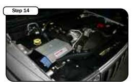
Place enclosed CARB EO sticker on a clean/smooth surface on or near the intake system. EO identification label is required in passing the Smoo Check Inspection. Your installation is now complete. Check all clamps and connections. Periodically check all clamps and hoses. Thank you for choosing afe!
