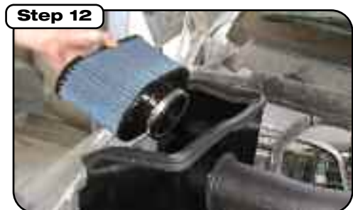
Attach filter to intake tube. It may be a tight fit, but DO NOT OIL OR GREASE TO INSTALL.
