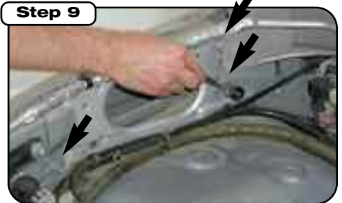
Remove three inner-fender bolts (13mm socket or wrench) for attachment of filter housing.
