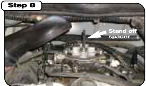
Install throttle cap stand off spacer (arrow) and cap. Reuse original throttle body gasket.
