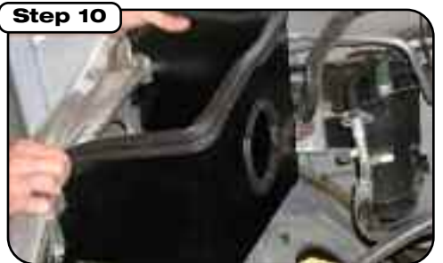
Install large housing trim seal to top of housing and small trim seal to tube inlet. Attach filter housing to inner fender-well with the three specified bolts.
