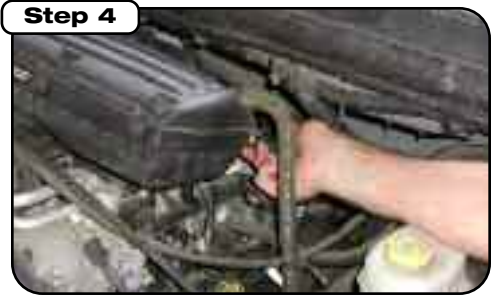
Loosen clamp at resonator box for throttle body and disconnect vent hose at valve cover.
