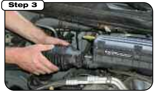
Remove air duct from resonator box and completely remove from engine compartment.
