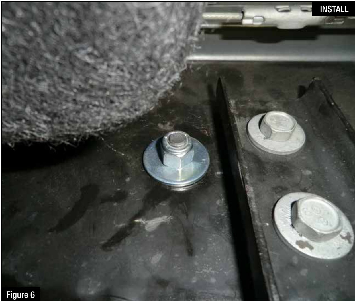
Step 7: Using the supplied 3/8" nut and washer, tighten the bracket on to the frame rail.
