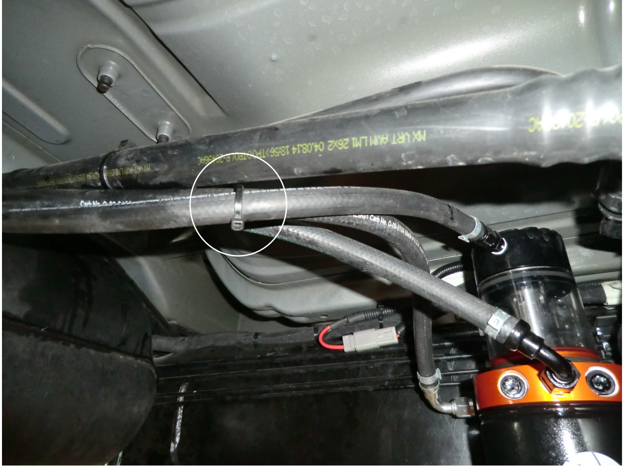
38. Route the hoses as shown and secure with the supplied nylon cable ties.
