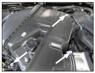
c. Loosen and remove the two 10mm bolts securing the airbox. Loosen the hose clamp on throttle body.
