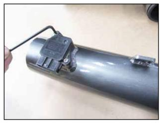
Install MAF sensor onto AEM upper tube(T) using the bolts(G) provided.
