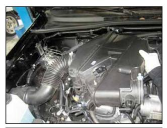
h. Disconnect air box from throttle and carefully remove stock assembly from the engine bay.
