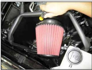
Install filter(U) onto air horn and secure with the provided hose clamp(A).
