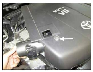
e. Check tube position by reinstalling engine cover and adjust until the bolt lines up to the engine cover as shown. Remove cover and tighten hose clamps once positioned in proper place.
