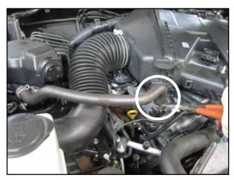
d. Loosen spring clamp and disconnect air pump hose as shown.
