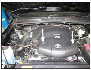
a. Stock intake system. Loosen the two nuts indicated to remove the engine cover.
