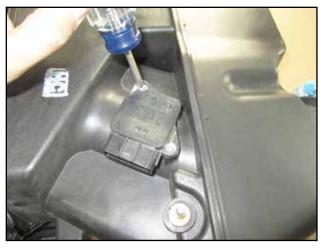
k. Remove the MAF sensore from the stock airbox and set aside for use with the AEM upper tube.
