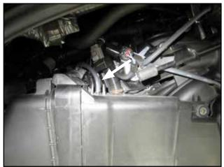
g. Disconnect fuel pressure regulator breather hose from the rear of the stock air box
