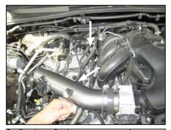
f. Replace fuel pressure regulator hose with the longer hose(V) provided and connect other end to the AEM tube(T) as shown.
