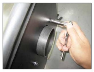
Mount air horn adapter(R) onto heat shield and secure with lock washers(E) and bolts(F) provided.
