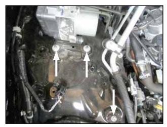
Remove the two nuts and one bolt indicated. Set aside for use later with AEM heat shield.
