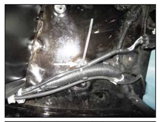
Provide adequate slack to pump harness and use zip tie(W) to secure harness to inner fender as shown. Trim excess end of zip tie.
