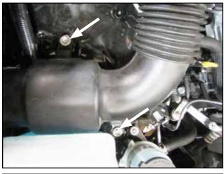
f. Remove the two bolts securing the stock intake inlet tube down.
