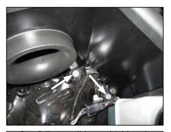
m. Carefully install heat shield and line up tabs to holes exposed in removal Step 2-i. Fasten lower tab near air horn using stock bolt from removal Step 2-f. Fasten tab near washer resevoir using bolt from removal Step 2-i. Reconnect air pump harness.
