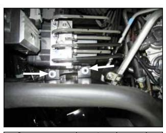
n. Secure rear tabs using the stock nuts from removal Step 2-i.
