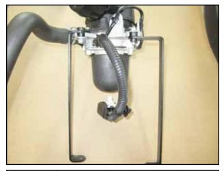
g. Loosely mount brackets(N,O) onto air pump as shown using provided bolts(H) and washers(J). Note: Short armed bracket is mounted on left side near hose as shown with bolt pointed upward.
