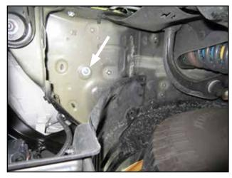
j. From under vehicle, install nut(I) and washer(J) onto bolt(H) previously installed. Check for clearance near washer reservoir and tighten nut.
