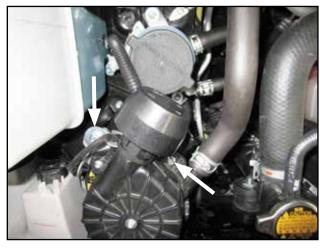
i. Re-install bolt removed in previous step to secure air pump bracket on right. Line up left bracket to inner fender hole and insert provided bolt(H) through bracket hole.
