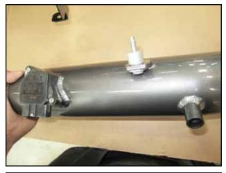
Use one bolt previously removed in removal Step 2-c and mount onto tab as shown using the provided aluminum bung(D).
