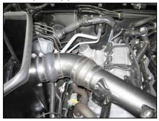
Ensure that hump hose is seated against heat shield and rotate lower tube into position. Tighten all four hose clamps.
