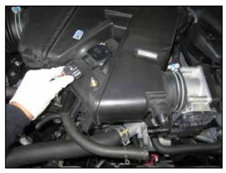
b. Loosen spring clamp to disconnect breather hose from plastic elbow.
