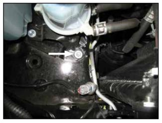
Remove the bolt indicated above on the power steering reservoir bracket and set aside for use in the next step.
