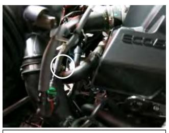
d. Loosen the hose clamp at the lower air intake tube.
