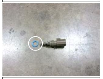
h. Remove the O-ring from air temperature sensor. Note: The O-ring will not be reused.
