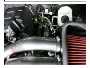
m. Connect the air temperature sensor connecter onto the air temperature sensor that was removed in step 2b.
