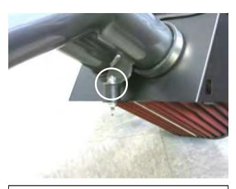
g. Install the provided nut and washer onto the AEM® intake tube bracket, then tighten both sides.
