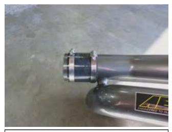
i. Install the straight coupler with hose clamps onto the AEM<sup>®</sup> tube. Note: Use soap and water to allow the coupler to slide on the intake tube.
