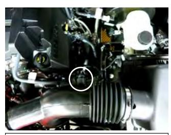
b. Disconnect the intake air temperature sensor connector.
