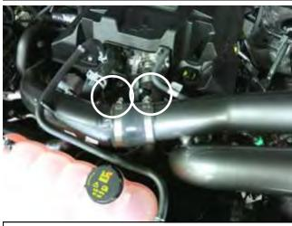
I. Install the straight coupler with hose clamps onto the stock upper intake tube. Tighten both hose clamps at this time.
