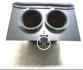
e. With the provided hardware, install the rubber mount/washer/nut onto the heat shield tab.
