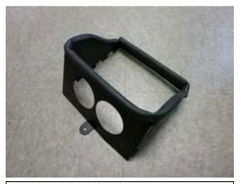
c. Install the provided edge trim onto the heat shield as shown. Note: Trimming the edge trim maybe necessary.
