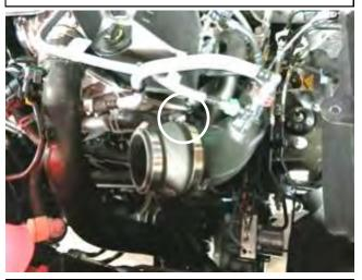
h. Install the step coupler with the provided hose clamps onto the lower intake tube as shown. Tighten hose clamp circled.
