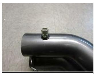
b. Install the air temperature sensor that was removed in step 2g into the AEM® intake tube.
