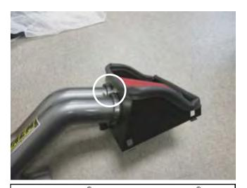
f. Install the AEM® intake tube into the AEM® air filter while aligning the rubber mount with the bracket on the intake tube. Tighten the hose clamps on the filter.
