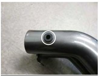
a. Install the provided grommet into the AEM® intake tube.
