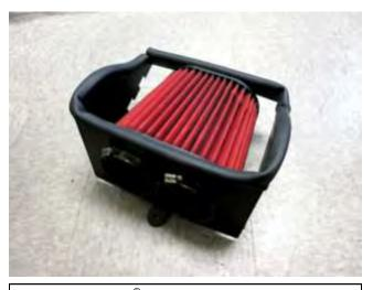
d. Install the  $\mathsf{AEM}^{\text{(8)}}$  filter into the heat shield with the provided hose clamps.
