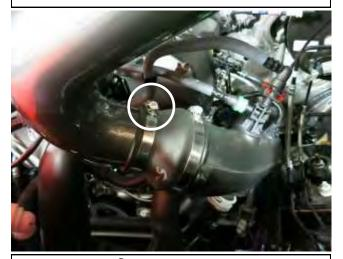
k. Align the AEM<sup>®</sup> intake tube with the step coupler that was previously installed in step 3h. Tighten the hose clamp circled at this time.
