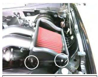
j. Install the assembled AEM<sup>®</sup> intake tube and heat shield into the vehicle. Align the heat shield into the lower air box and latch the clips to secure it in place.
