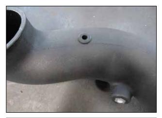
o. Install the supplied grommet (784642) into the AEM  $^{\mbox{\tiny @}}$  intake tube (9-0402).
