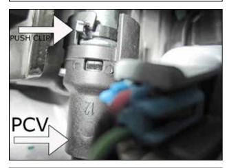
g. Release the PCV line from the engine by rotating it to the right and pushing the clip to the side.
