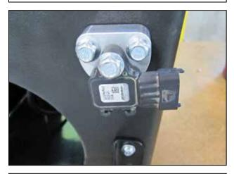
f. Install the filter minder sensor onto the adapter using 1 M6 bolt (1-2038).
