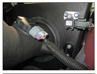
z. Reconnect the MAF air flow sensor and filter minder sensor.
