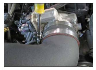
u. Tighten the hose clamp (9464) at the throttle body.
