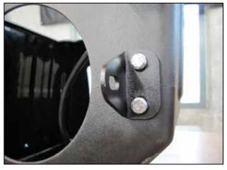
c. Install the pipe bracket (32-3079) onto the AEM<sup>®</sup> air box (9-0390-1) using the supplied M6 bolts (1-2065) and washers (1-3016).
