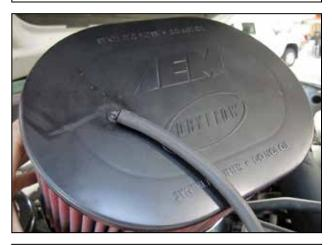
q. Attach the filter minder hose (5-3020) to the 90° fitting (8-152).
