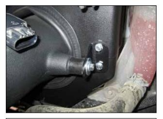
t. Install the rubber mount (1228599-1), washer (08160) and M6 nut (444.460.04) onto the bracket. Align for best fit and tighten the bracket bolts and rubber mount.
