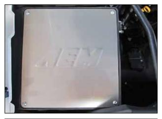
y. Install the AEM<sup>®</sup> air box lid (20-8514) using the 4 M6 bolts (1-112) and nylon washers (1-3001).
