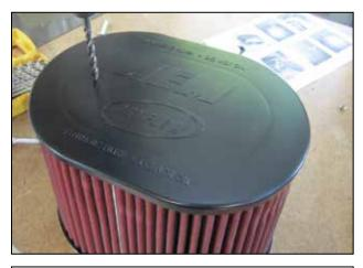
j. Drill a 1/4" hole in the filter cap of the air filter (21-2277DK), below the corner of the "A" for the filter minder grommet.
