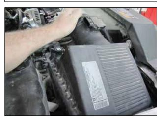
j. Remove the air box from the vehicle by firmly lifting up to disengage it's clips.
