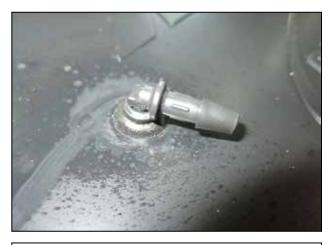
k. Install the grommet (784631) and 90 deg. fitting (8-152) into the air filter's filter cap as shown.
