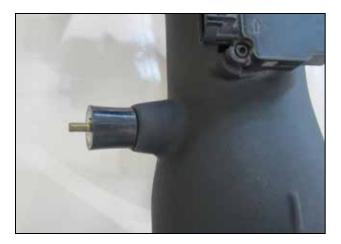
n. Attach the supplied rubber mount to the set screw supplied and install it 3/8" away from the rubber and then thread it into the AEM<sup>®</sup> intake tube (9-0402).
