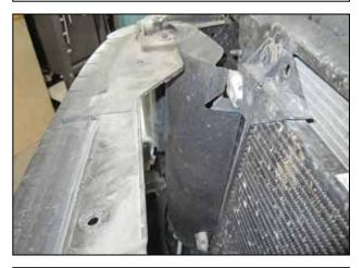
n. Locate the air deflector behind the grill on the passenger side of the radiator.
