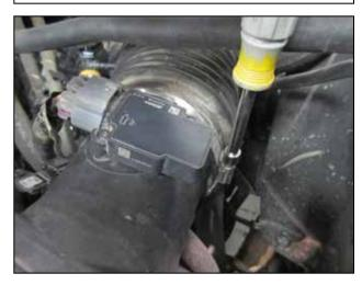
d. Loosen the hose clamp at the air box neck.
