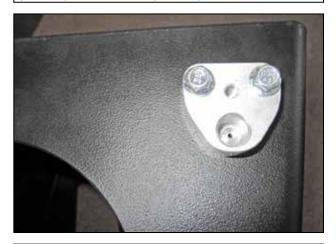
e. Feed the hose (5-3020) through the hole and mount the adapter (2-604) to the air box (9-0390-1) using 2 M6 bolts (1-2038).
