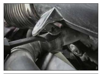
e. Unclip the radiator hose from the intake tube.
