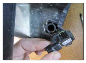
s. Remove the filter minder sensor from the air box.
