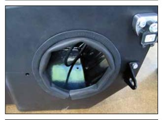
g. Install the rubber edge trim (8-4018) onto the AEM $^{\circ}$  air box (9-0390-1) as shown.
