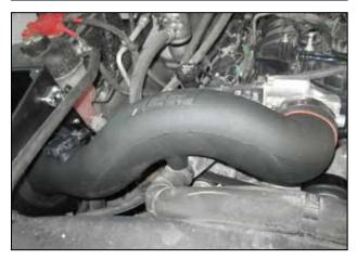
p. Install the AEM® intake tube (9-0402) as shown.
