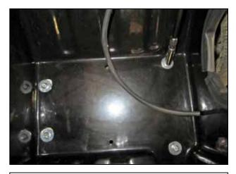
i. Secure the AEM<sup>®</sup> air box (9-0390-1) using the 4 supplied M6 bolts (1-2038) and washers (08160).
