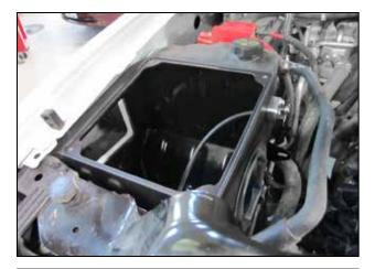
h. Install the AEM<sup>®</sup> air box (9-0390-1) into the vehicle.
