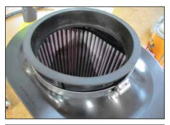
I. Install the filter adapter (5-1051) and #80 hose clamp (103-BLO-8020N) on the air filter (21-2277DK) as shown.
