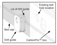
D. Start at front of box, use square hole to slide u-nut on CarbonPro™ box until extended threads align with existing bolt hole location.
