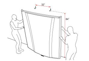
Before removing the cover (A), mount the two J-Hooks (I) with the mounting screws (J) provided, on the garage wall. The hooks must have a minimum height from the floor of 84". Center horizontally 32" apart from each other. For long bed trucks mount 98" from the floor. Then remove the cover from the truck bed.
