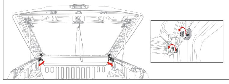
**11 Final adjustments.** Be sure the front flap hangs over the bulkhead of the truck. The latch strike can be adjusted by loosening the two nuts and moving the strike up or down to make better contact with the latch. The rotary latch can be adjusted by loosening the two nuts and moving the latch in or out to make better contact with the strike.
