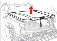
Next, pull the cover (A) rearward, releasing the hinge from the mounting brackets (B & C), and lift the cover off.
