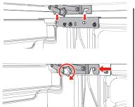
Slide the slots in the 4 bar hinges (attached to the cover) over the posts on the front mounting brackets. Then push the cover forward to lock the hinges to the mounting brackets.
