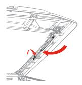
Place the loose end of the strut (D) in the storage clip. Repeat on the opposite side.
