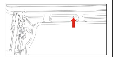
Finally, hang the cover vertically by locating the two holes on the underside of the cover. With the cover facing away from the wall, carefully align the holes in the cover with the hooks on the wall. Gently lift the cover and slide the hooks through the holes until they are fully inserted.
