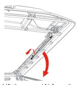
Lift the cover (A) from the rear and tighten the twist knobs (K) on both left and right hinges.
