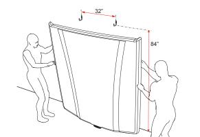
Before removing the cover (A), mount the two J-Hooks (J) with the mounting screws (Kw) provided, on the garage wall. The hooks must have a minimum height from the floor of 84". Center horizontally 32" apart from each other. For long bed trucks mount 98" from the floor. Then remove the cover from the truck bed.
