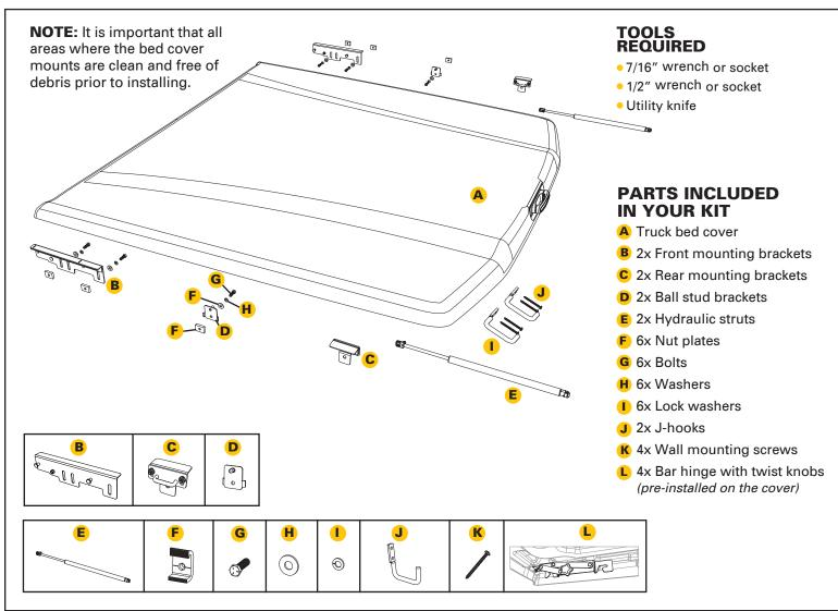
1 If NO plastic drop-in bedliner is present, skip to step 2. Trucks that have plastic drop-in bedliners will require some minor trimming of the bedliner to ensure proper placement of the mounting brackets (B & C).
