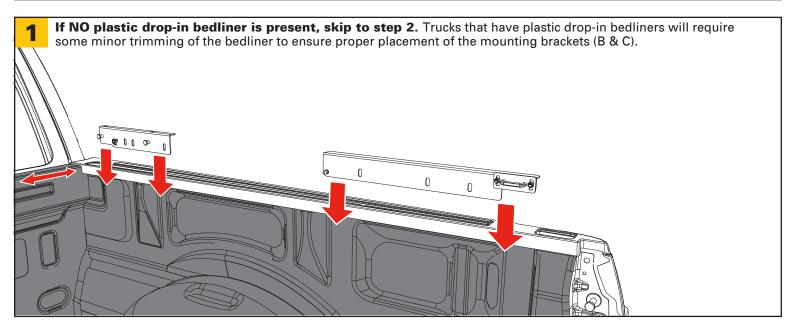
REAR mounting brackets. The rear bracket (B) should be installed on the truck bed rail near the tailgate. To determine the exact location, measure from the back side of the bulkhead to the front edge of the bracket. The specific dimensions for your vehicle can be found on the measurement chart located on the back page of this instruction manual.
