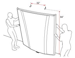
Before removing the cover (A), mount the two J-Hooks (I) with the mounting screws (J) provided, on the garage wall. The hooks must have a minimum height from the floor of 84". Center horizontally 32" apart from each other. For long bed trucks mount 98" from the floor. Then remove the cover from the truck bed.
