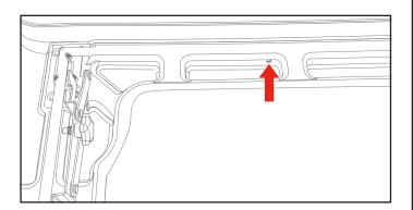
Finally, hang the cover vertically by locating the two holes on the underside of the cover. With the cover facing away from the wall, carefully align the holes in the cover with the hooks on the wall. Gently lift the cover and slide the hooks through the holes until they are fully inserted.
