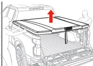
Next, pull the cover (A) rearward, releasing the hinge from the mounting brackets (B & C), and lift the cover off.
