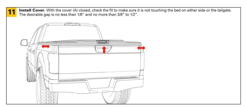
Install Cover. To adjust the cover (A) from front to back to be more even, loosen the clamps (E) and move both of the front brackets (C) forward or rearward accordingly. To adjust to one side or the other, move the front brackets forward or rearward independently. Retighten all of the clamps.
