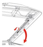
Lift the cover (A) from the rear and tighten the twist knobs (L) on both left and right hinges.
