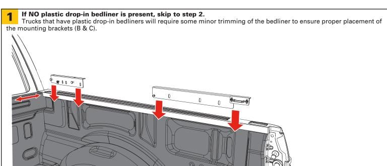
REAR mounting brackets. The rear bracket (B) should be installed on the truck bed rail near the tailgate. To determine the exact location, measure from the back side of the bulkhead to the front edge of the bracket. The specific dimensions for your vehicle can be found on the measurement chart located on the back page of this instruction manual.
