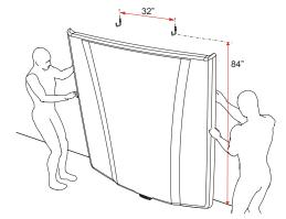
Before removing the cover (A), mount the two J-Hooks (J) with the mounting screws (K) provided, on the garage wall. The hooks must have a minimum height from the floor of 84". Center horizontally 32" apart from each other. For long bed trucks mount 98" from the floor. Then remove the cover from the truck bed.
