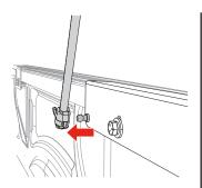
Release the strut (D) off of the ball stud, and be sure to secure the cover (A) to prevent it from closing unexpectedly.
