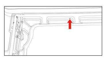
Finally, hang the cover vertically by locating the two holes on the underside of the cover. With the cover facing away from the wall, carefully align the holes in the cover with the hooks on the wall. Gently lift the cover and slide the hooks through the holes until they are fully inserted.
