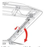
Lift the cover (A) from the rear and tighten the twist knobs (K) on both left and right hinges.
