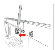
Release the strut (D) off of the ball stud, and be sure to secure the cover (A) to prevent it from closing unexpectedly.
