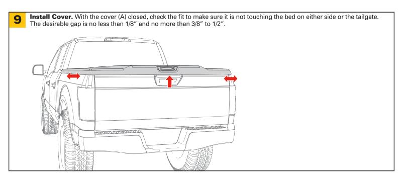
Install Cover. To adjust the cover (A) from front to back to be more even, loosen the clamps (E) and move both of the front brackets (C) forward or rearward accordingly. To adjust to one side or the other, move the front brackets forward or rearward independently. Retighten all of the clamps.
