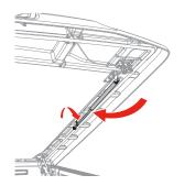
Place the loose end of the strut (D) in the storage clip. Repeat on the opposite side.
