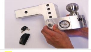
STEP 4: Pull on the <u>Key Lock Assembly</u> to ensure that it has engaged and place the <u>Dust Lock Cover (E)</u> over the lock. Do not operate without making sure the <u>Key Lock Assembly</u> is securely locked in place.
