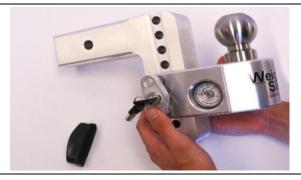
STEP 3: Once you have achieved the desired position along the <u>Drawbar</u>, insert the <u>Key Lock Assembly (D)</u> into the <u>Weigh Safe Slider</u> and lock in place by turning the key.
