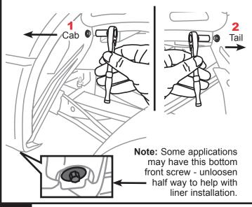
6 Start on the driver side by setting the driver side wheel well (A) marked as (DS) inside the inner panel of the truck's wheel
