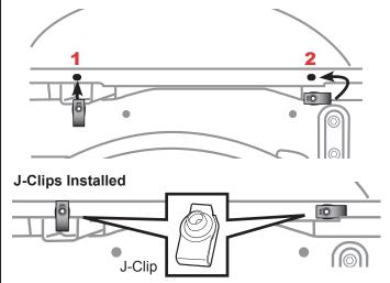
Tuck the bottom sides of the lower part of the wheel well liner behind the metal lip of truck's fender and then tuck the upper part. Then install two screws (D) provided in places 1 & 2 using a ratchet with 10mm socket. After that re-install the two fasteners saved in step 4 in places 3 & 4.
