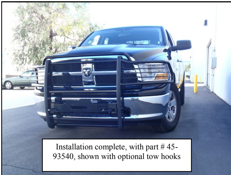
Installation complete, shown with optional stainless steel faceplate and tow hooks
