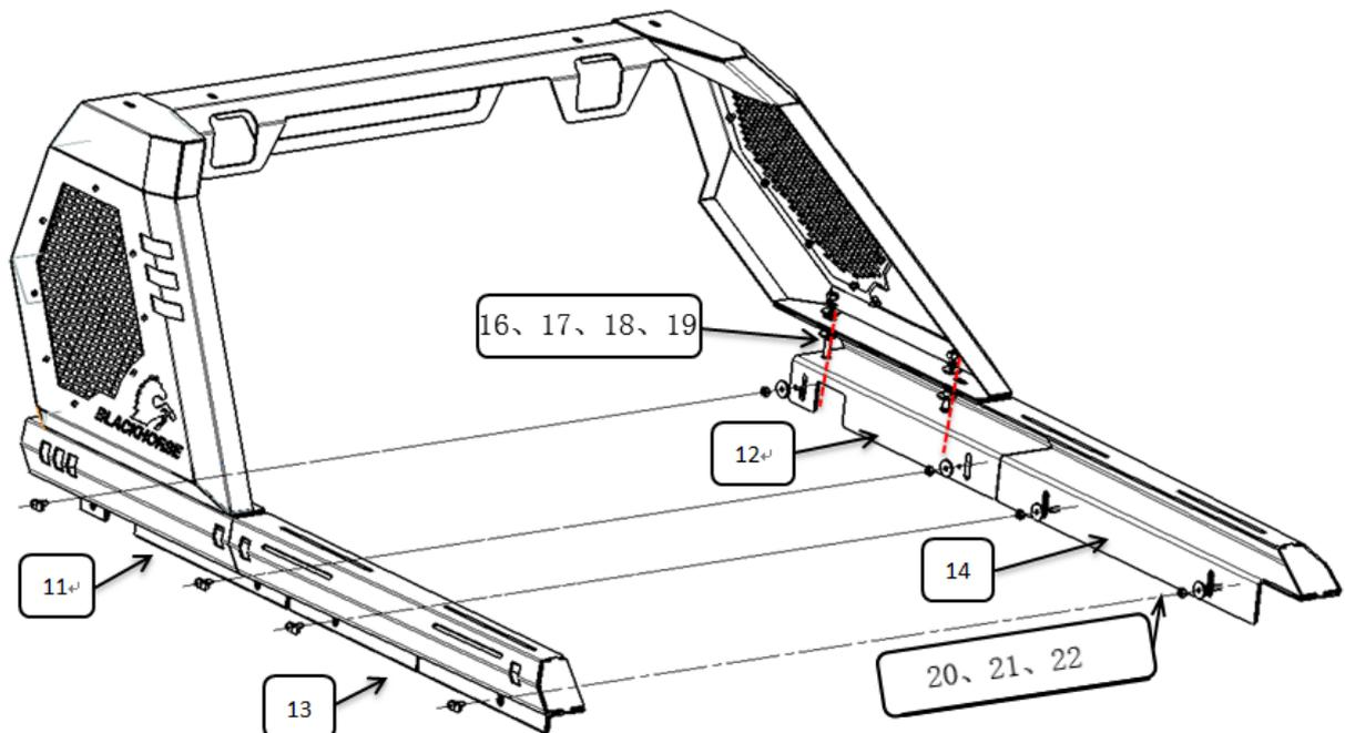
**Step 4:** Test and make sure that the roll bar is steadily fixed, fully tighten all hardware.
