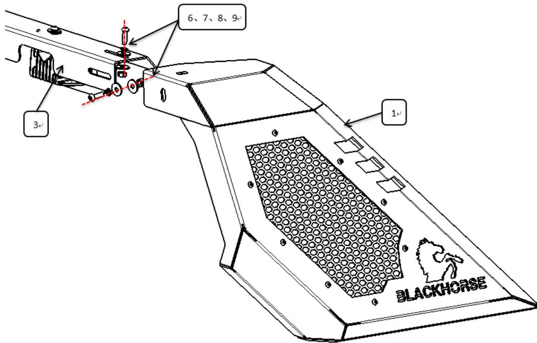
**Step 3:** Connect brackets and roll bar with standard parts ⑩ ⑪ ⑫ ⑬ as figure shows.
