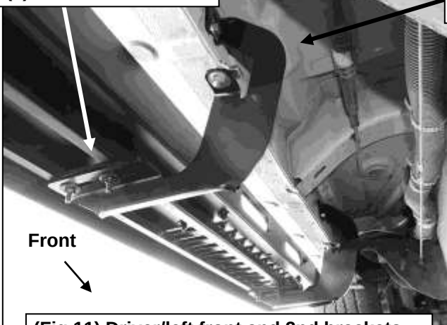
(Fig 11) Driver/left front and 2nd brackets
