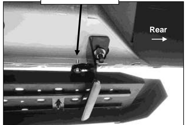
(Fig 26) Passenger/right rear Bracket installation
