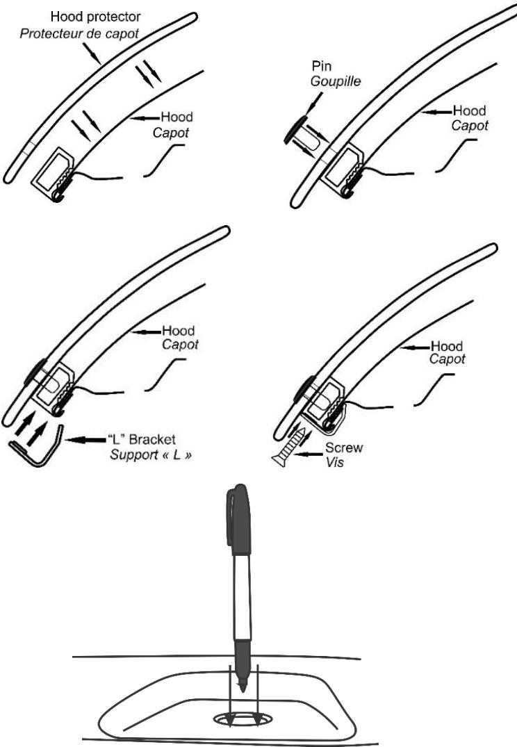
6. With the hood protector in place, assemble the four pieces of the hood edge clip (see illustrations) and loosely attach it to the edge of the hood. Ensure the hood protector is centered and tighten the screws into the clips.
