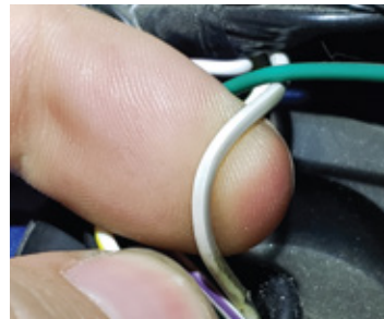
Jeep Wrangler JK 12V Power Location (White/Grey wire by passenger kick panel)
