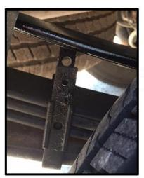
Remove rear clip bolt and roller on Titan models that are attached with a removable nut and bolt. Do not remove bracket.
