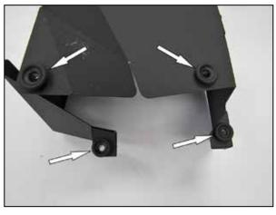
5. Remove the four mounting grommets from the factory air filter housing and install them into the SPECTRE® heat shield as shown.
