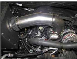
11. Install the SPECTRE® intake tube into the flex coupler and then onto the throttle body, adjust the tube for best fit and then secure with the provided hose clamps.
