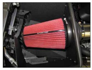
13. Install the SPECTRE  $^{\! \rm B}$  air filter and secure with the provided hose clamp.
