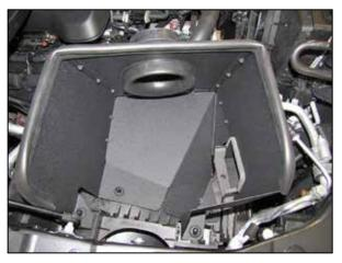
8. Install the heat shield into position as shown.
