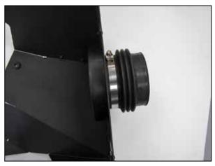
6. Install the filter adapter and flex coupler as shown and secure with the provided hose clamp.
