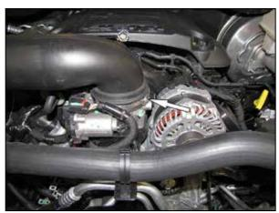
3. Loosen the hose clamp at the throttle body and then lift the complete intake system out of the vehicle.
