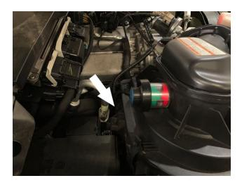
Lift up the stock intake box slightly to unseat the prongs from the stock grommets, then remove the stock intake box from the vehicle.
