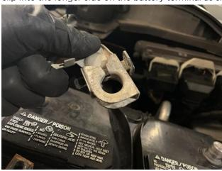
Reinstall the tightening mechanism and then flip the negative cable terminal over. The longer side of the negative battery terminal should be facing the passenger side during installation. Open up the battery terminal diameter by opening up the slit with a screwdriver so it will be easier to get the terminal fully seated onto the battery post.
