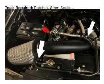
Attach the provided MAF harness extension (Q) to the existing MAF sensor connector by inserting the male end and engaging the red locking clip.
