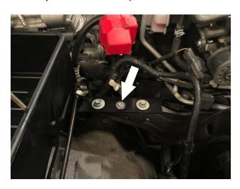
Reattach the grounding bolt removed in Step 19 as shown. Re-use the factory grounding bolt to attach the primary ground to it's original threaded hole on the fender and torque to factory specifications, 106 lb-in (12Nm). Note: The primary ground should be at an angle with the prong facing away from the fender as shown.
