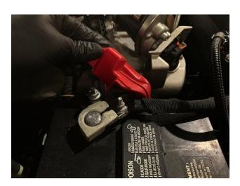
Place the positive terminal cover over the positive terminal and verify that the battery cables and extensions are as close as possible to the side of the battery so that all cables and wires are away from any hot components or moving parts that could potentially damage the cables or wires.
