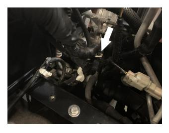
Install the provided grommet into the hole on the intake tube support bracket.
