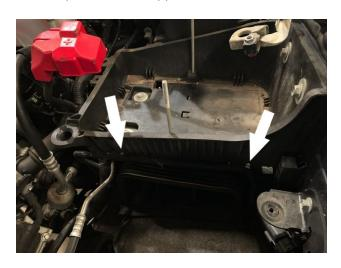
Remove the four screws then remove the battery tray from the vehicle. Set the screws aside, they will be reused in Step 15.
