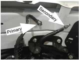
Remove the grounding bolt that attaches the primary ground to the fender. Set the grounding bolt aside to be used in Step 23.
