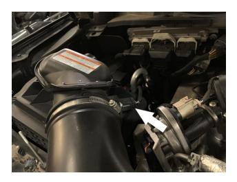
Disconnect the hoses attached to the stock intake tube.
