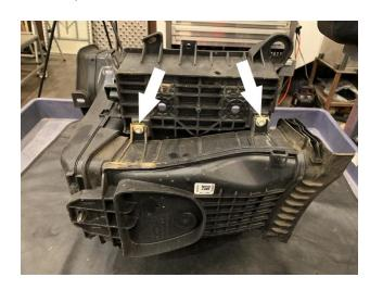
Push the locking tabs and lift the stock inlet away from the stock battery tray.
