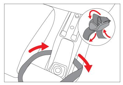
3. Slip side strap between seat belt and front pillar. Hook end of strap to front pillar so hook is level with tonneau extension. Pull end of strap to tighten.
