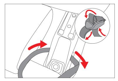
3. Slip side strap between seat belt and front pillar. Hook end of strap to front pillar so hook is level with tonneau extension. Pull end of strap to tighten.
