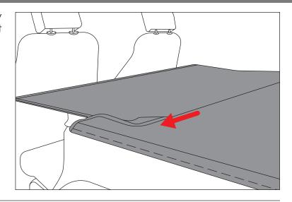
2. Wrap long straps on tonneau extension under seat brackets, thread each strap end through buckle, and tighten straps.
