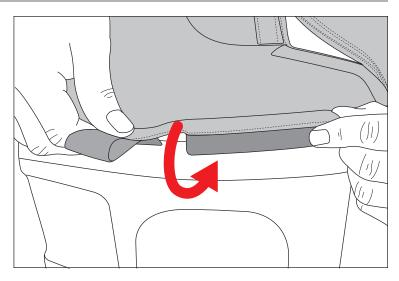
6. Wrap collars around rear sport bar and fasten hook and loop strips together. Repeat for opposite side.
