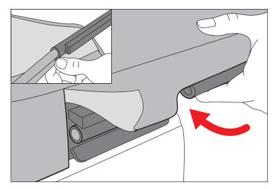
3. Zip Windbreaker to tonneau cover using zipper under flap of Windbreaker. Complete Winbreaker installation before proceeding.
