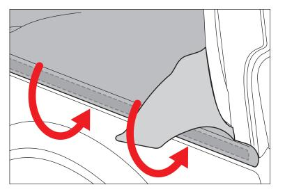
5. Roll plastic strip over edge and into rear groove of body tub. Repeat for opposide side.
