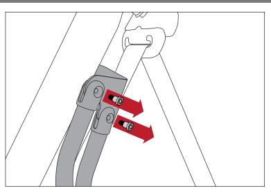
2. Remove tailgate bar from soft top. Insert tailgate bar on tubed strip of tonneau cover and into tailgate mounts on each side of tailgate opening.
