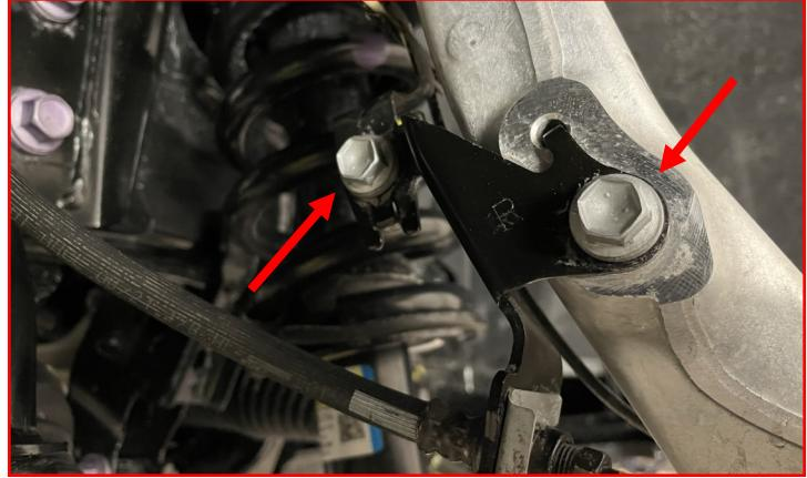
Remove the **ABS wire bracket** at the bottom of the knuckle.
