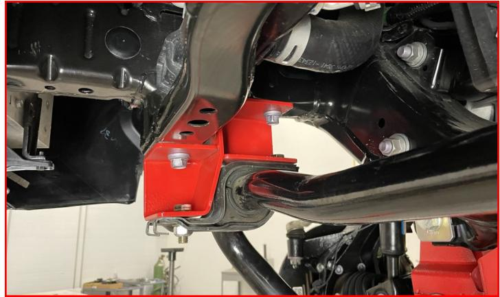
Install the supplied skid plate using the **supplied 3/8-16 X 1" hex head bolts, lock nuts, and flat washers**.
