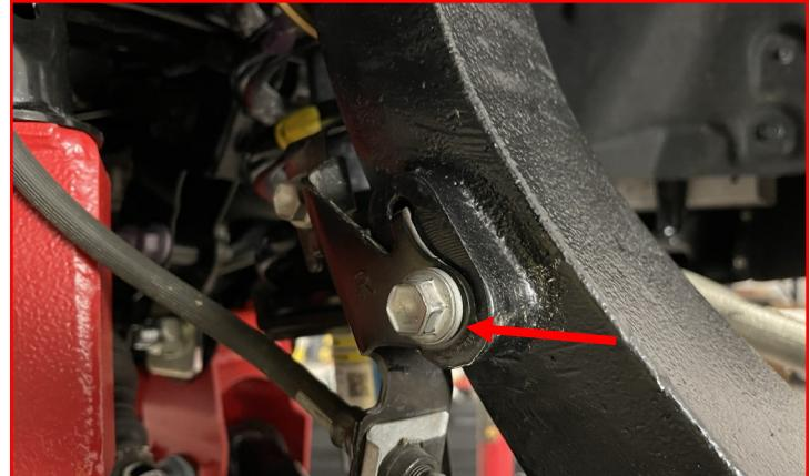
Using **factory hardware**, attach the ABS sensor wire at the bottom of the knuckle.
