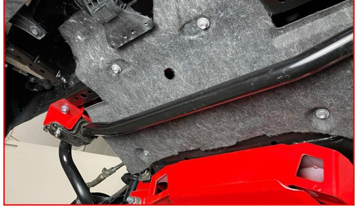
Trim the front air dam 0.25" from the inner edge. Contour the line to blend it into the air dam.
