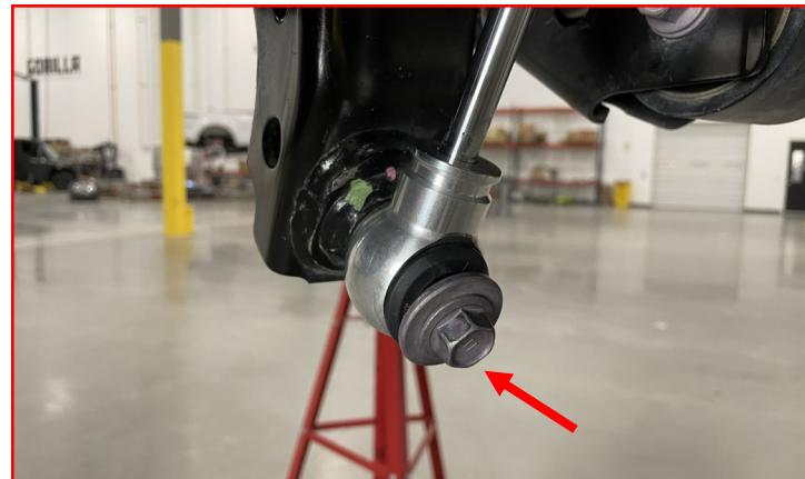
Using the **supplied shock hardware**, attach the shock to the upper mount.
