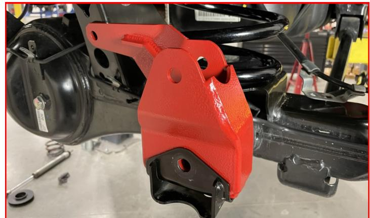
Using **factory hardware**, attach the bracket to the axle in the factory mounting location.
