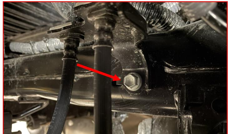
Remove the **bolt** holding the brake line to the axle.
