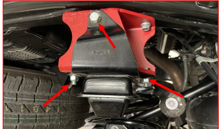
Attach the **supplied rear shock** to the lower mount using **factory hardware**.
