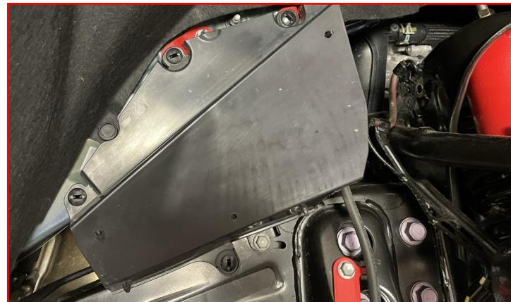
Using **factory hardware**, install the front **sway bar drop brackets**. Note that they are handed with the pockets facing inboard and the smaller mating faces towards the front of the vehicle.
