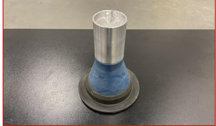
Attach the supplied bump stop extension to the factory isolator using thread locker and the supplied **M10-1.5 X 25mm hex bolt and M10 washer**.
