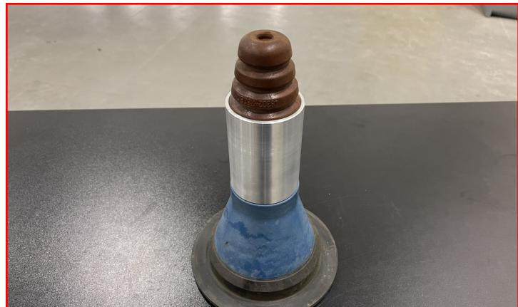
Place the factory bump stop and isolator on the top of the spring as shown.
