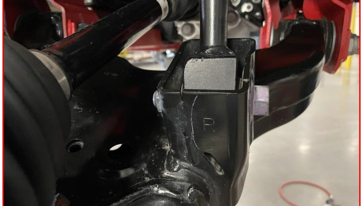
Remove the **four (4) factory bolts** holding the knuckle to the hub.
