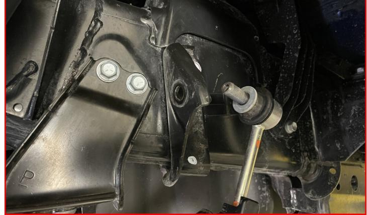
Remove the **Panhard bar bolt** at the axle and let it rest in the mounting perch.
