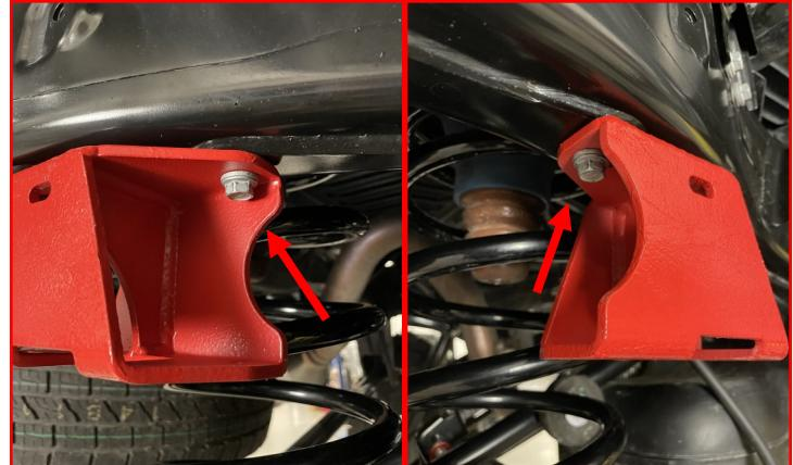
Attach the factory bump stop to the extension using the supplied M8-1.25 X 20mm hex head bolts and M8 flat washers, starting with the lower bolts.
