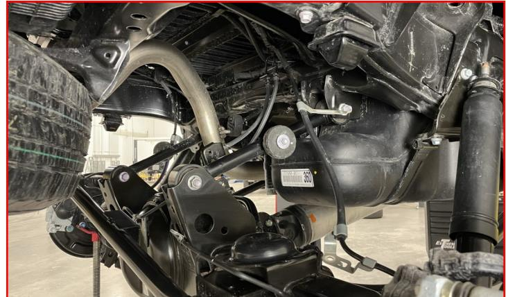
Remove the factory bump stop from the factory spring isolator.
