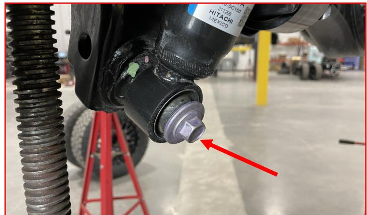
Remove the **upper shock nut** and **bushing**.
