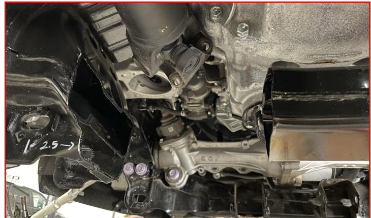
Temporally install the **rear crossmember** with the differential mount on the driver side. Use the **supplied M18-2.5 X 160mm hex heads bolts** and **cam block off plates** (four total).
