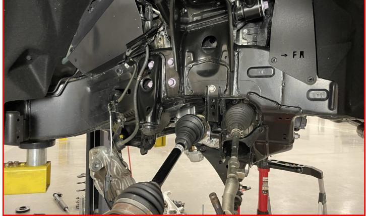
Remove the **four (4) nuts** holding the drive shaft to the front differential.
