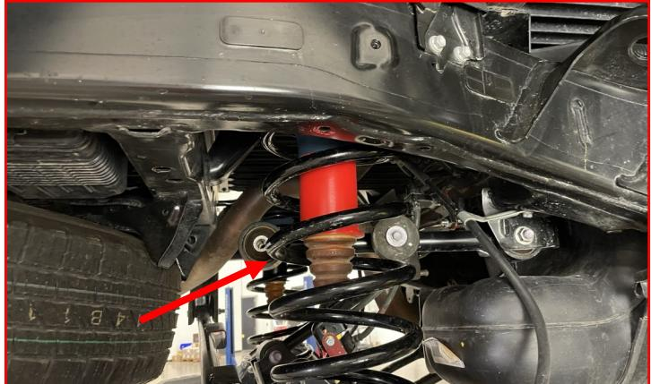
Install the **PASSENGER** upper control using **factory hardware**. **DO NOT** tighten at this time.
