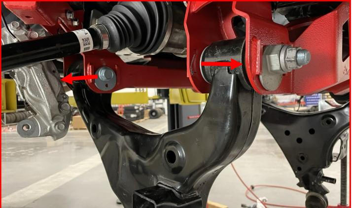
Remove the factory bump stop from the chassis mount.
