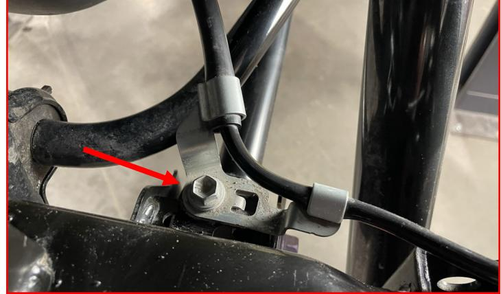
Remove the **bolt** (one on each side) holding the brake line to the body.
