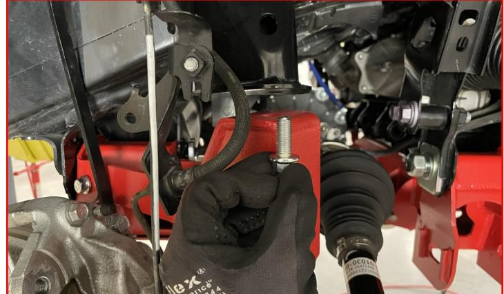
Feed a ratchet extension up through the lower mounting hole to tighten the bolt.
