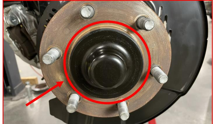
Remove the **cotter pin**, **sleeve**, and **nut**.
