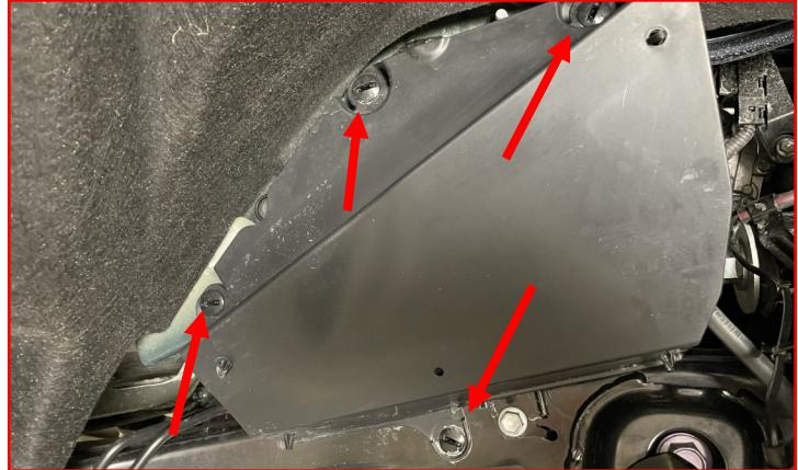
Remove the rear cover for caliper hanger hole.
