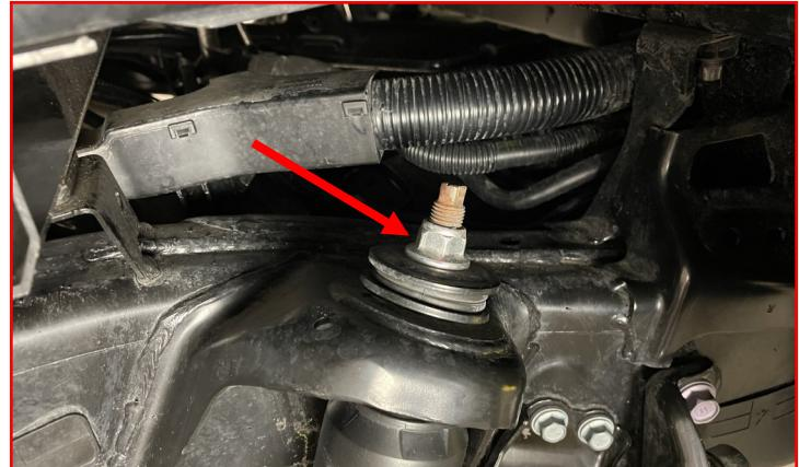
Lower the axle enough to remove the **rear springs**.
