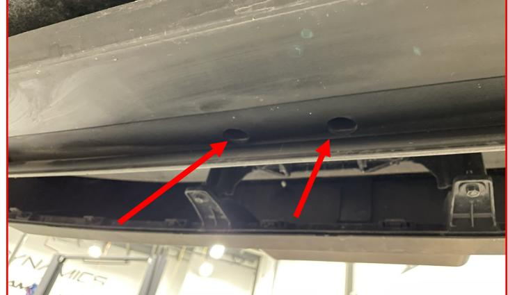
Remove the four (4) bolts for the **front dust shield**.
