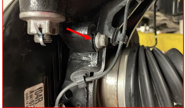
Using **factory hardware**, attach the ABS/wheel speed sensor.
