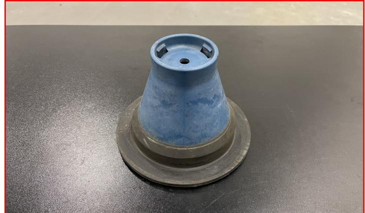
Install the supplied rear bump stop extension onto the factory isolator.
